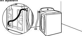
Floor drain system requires a Siphon Break Kit (Part Number 285834), 2 Connector Kits (Part Number 285835), and an Extension Drain Hose (Part Number 285863) that may be purchased separately. To order, please see toll-free phone numbers in your Use and Care Guide. Minimum siphon break: 28" (710 mm) from bottom of washer. (Additional hoses may be needed.)
